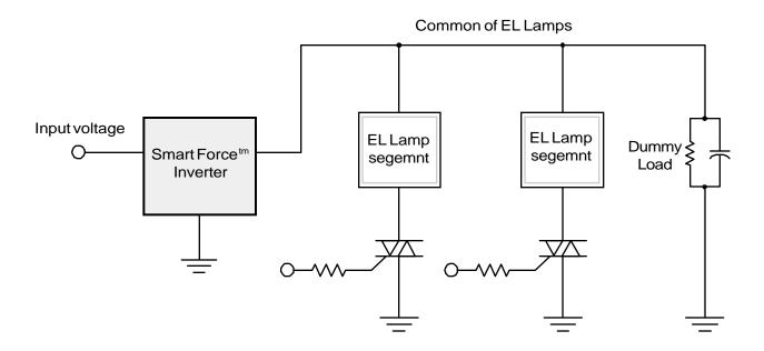
Figure 9. El lamp segment switching, first quadrant
