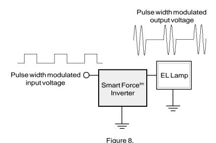
Pulse width modulated dimming
