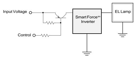
Figure 3. Input switching using a PNP transistor
