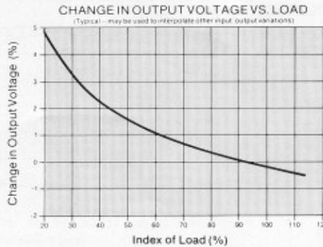
**E1200 DC-DC Converters, Unregulated, Single Output only for High Voltage Displays, Charging Capacitor Banks and other applications requiring up to 25W total output power!**
