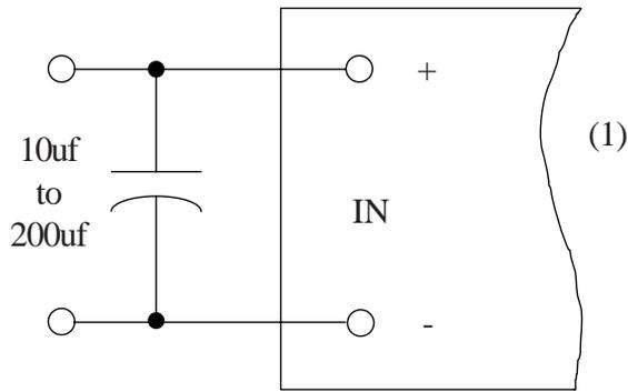
These filtering configurations will minimize the amount of switching ripple reflected on the DC input.
