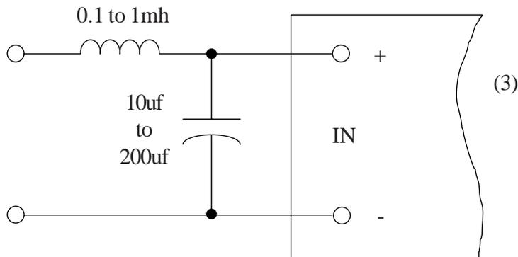
Figure (3) provides adequate input filtering for analog systems.
