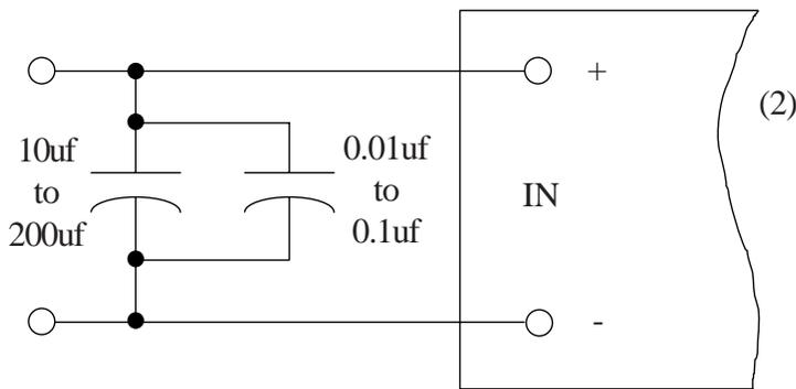
These filtering configurations will minimize the amount of switching ripple reflected on the DC input.
